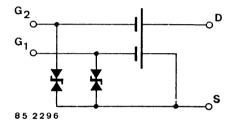
BF961 Marking Plastic case (~TO 50) 1 = Drain, 2 = Source, 3 = Gate 1, 4 = Gate 2 BF961 Marking Plastic case (~TO 50) 1 = Drain, 2 = Source, 3 = Gate 1, 4 = Gate 2
